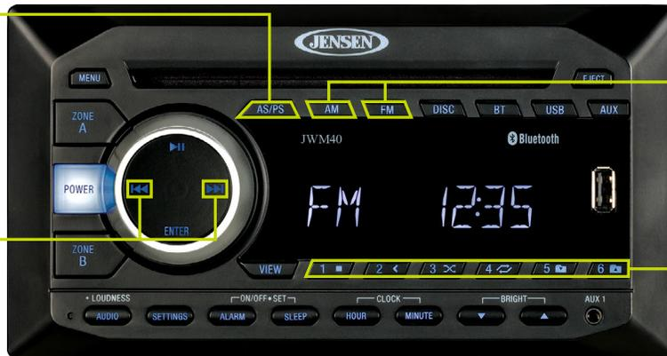
**MODE/BAND:** Press to access TUNER mode and that particular band. Press AM button repeatedly to select band AM1 or AM2. Press FM button repeatedly to select band FM1, FM2 or FM3.
